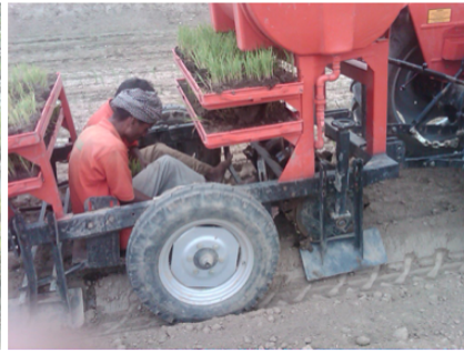
Transplanting rice seedling with water wheel transplanter in dry soil
