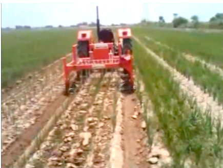
Once the seedlings were established, a Precision Weeder-Aerator device reduced weed growth.
