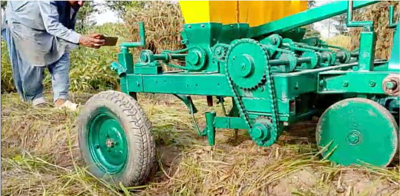
Five row tractor mounted VIPP - mechanical
